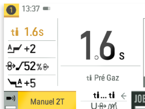
Settings: Pre-gas, I Start, Wire creep, Burn Back, Post-gas
